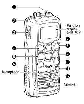
Sub-microphone (p. iii) ANTENNA CONNECTOR (p. 2) Connects the supplied antenna.
