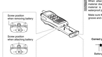
**NOTE:** When removing or attaching the battery pack, use a coin or standard screwdriver to loosen or tighten the bottom screw.
