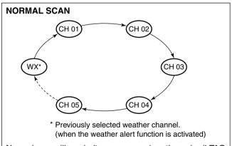
Normal scan, like priority scan, searches through all TAG channels in sequence. However, unlike priority scan, Channel 16 is not checked unless Channel 16 is set as a TAG channel.
