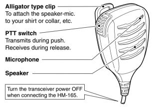
**NEVER** immerse the connector in water. If the connector gets wet, be sure to dry it BEFORE attaching it to the transceiver.
