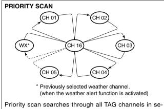
quence while monitoring Channel 16. When a signal is detected on Channel 16, scan pauses until the signal disappears; when a signal is detected on a channel other than Channel 16, scan becomes Dualwatch until the signal disappears. Set the TAG channels (scanned channels) before scanning. Clear the TAG for unwanted channels which inconveniently stop scanning, such as those for digital communications. (p. 15)
